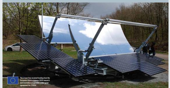
The co-generated heat is conducted through the aluminium pipe to the heat transfer fluid (water, water with glycol or potentially thermal oil) circulating in the tube. This fluid cools the cells and transports the heat to the user or the storage. Altogether, the receiver reaches up to 30% electric efficiency and 45% thermal efficiency in relation to the direct radiation, representing one of the highest solar efficiencies worldwide.
