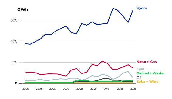
Figure 1: Sources of Colombia's electricity generation
