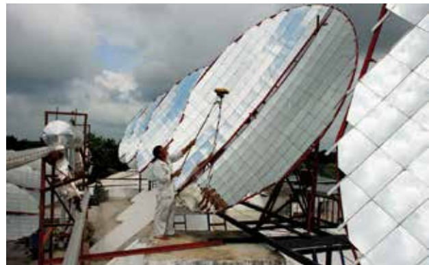
The agricultural college at the Muni Seva Ashram in India cooks for its 500 students using steam produced by ten solar cookers.
